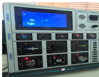
Figure 7. Schematic of the AI module with camera and LED indicator.
